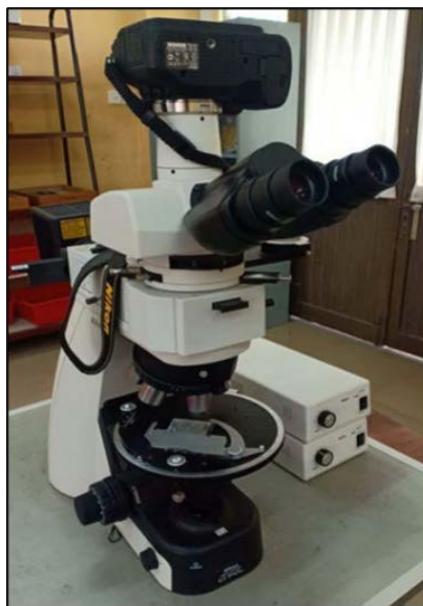
Figure 3.4: Nikon ECLIPSE Ci-POL use to analyse minerals and fossils content.
