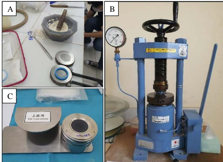
Figure 3.5: (A) Grinding samples, (B) Pressing the sample with hydraulic press machine, (C) Prepared samples.
