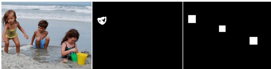
Figure 3.19. Comparison results between HOG and CNN-based face detectors. (first image) Input image, (second image) result of HOG-based face detector, and (last image) result of CNN-based face detector.
