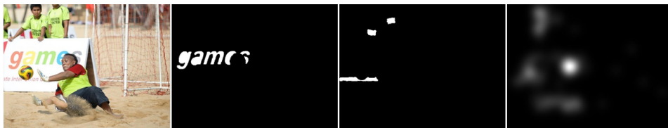
Figure 3.11. Our defining big and small text features and eye-tracking fixation map from the OSIE dataset. (first image) Input image, (second image) big text features, (third image) small text features, and (last image) eye-tracking fixation map.
