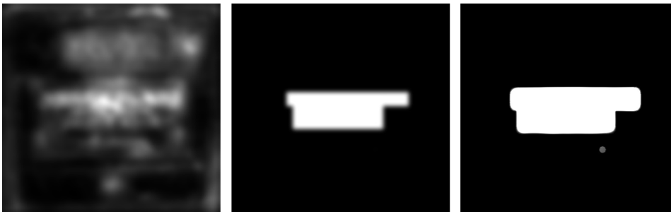
Figure 3.6. An example result of multiplication between saliency map and text detection. (first image) result of saliency map, (second image) result of Gaussian filtering on text detection, (last image) result of multiplication.
