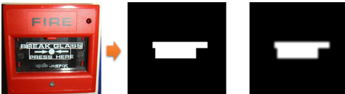
Figure 3.3. An example result of black and white and Gaussian filtering. (first image) Result of text detection, (second image) result of black and white filtering that white area is detection, and black area is background, (last image) result of Gaussian filtering.
