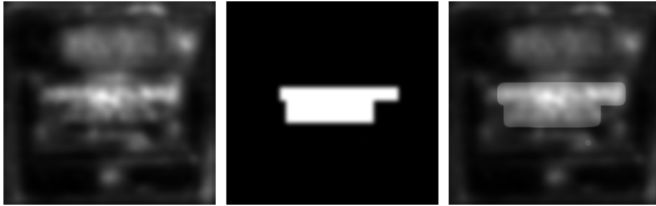
Figure 3.7. An example result of weighting between saliency map and text detection. (first image) result of saliency map, (second image) result of Gaussian filtering on text detection, (last image) result of weighting.
