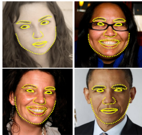
Figure 2.9. Selected results on the HELEN dataset. An ensemble of randomized regression trees is used to detect 194 landmarks on face from a single image in a millisecond.
