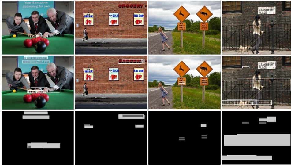
Figure 3.14. Applying a traditional text detection method. (first row) Input images, (second row) result of text detection inside white bounding boxes, and (last row) converting text detection areas into white to indicate text features. The results contain both big (brighter) and small texts.
